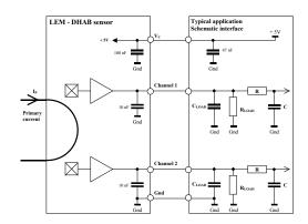
$\mathbf{R}_{L} > 10 \text{ k}\Omega$  optional resistor for signal line diagnosis  $\mathbf{C}_{L} < 100 \text{ nF}$  EMC protection RC Low pass filter EMC protection (optional)
